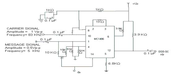
Fig.1.Balanced Modulator Circuit
