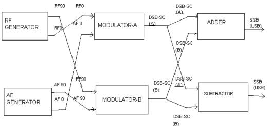
Fig.1Single Side Band system
